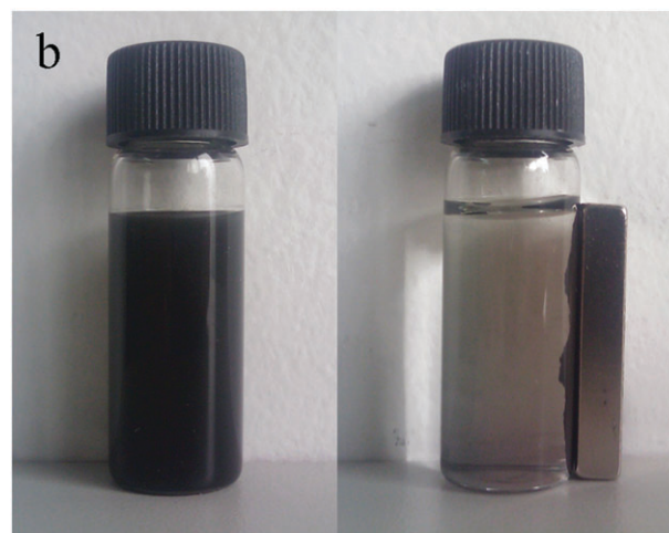
Fig. 6 (a) Room-temperature magnetization hysteresis loops of graphene/ \text{Fe}_3\text{O}_4 composites with a starting \text{FeCl}_3 \cdot 6\text{H}_2\text{O} amount of 0.5 g. (b) The behaviour of the composites under an external magnetic field.
